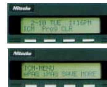
Soft Key Display Example While Placing ICM Call (to a Busy Station)
